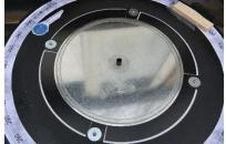
Early trials of the push too arrangement were disappointing and it was realised that the telescope needed to be levelled to achieve consistent and accurate results.
